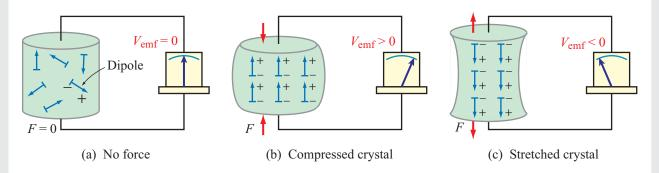
Figure TF12-1: Response of a piezoelectric crystal to an applied force.
