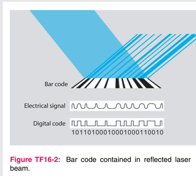
**Figure TF16-2:** Bar code contained in reflected laser beam.
