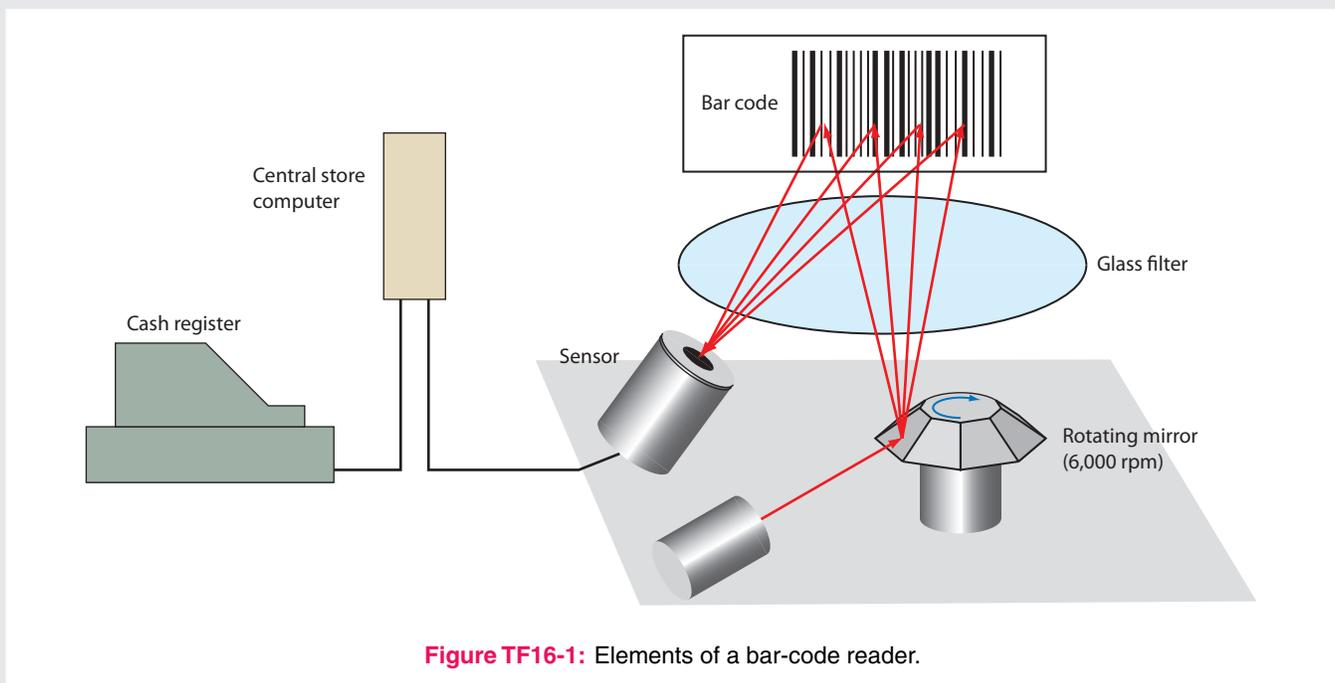
**Figure TF16-1:** Elements of a bar-code reader.
