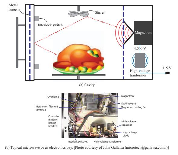
Figure TF3-2: (a) Microwave oven cavity and (b) electronics bay.
