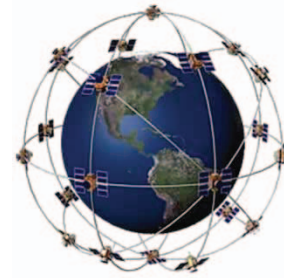
Figure TF5-2: GPS nominal satellite constellation. Four satellites in each plane, 20,200 km altitudes, 55° inclination.
