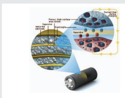
**Figure TF8-1:** Cross-sectional view of an electrochemical double-layer capacitor (EDLC), otherwise known as a supercapacitor. (Courtesy of Ultracapacitor.org.)
