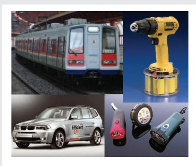
Figure TF8-2: Examples of systems that use supercapacitors.
