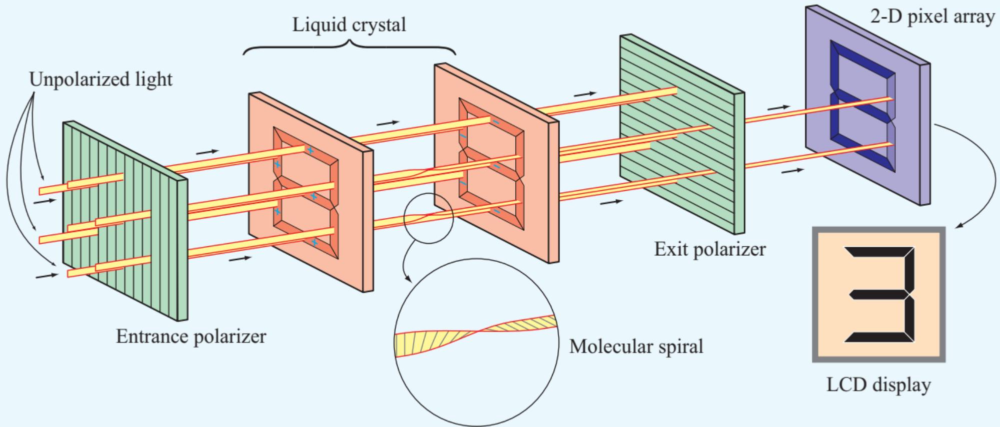
**Figure 1-1** 2-D LCD array.
