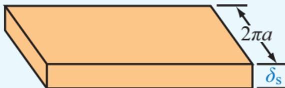
(b) Equivalent inner conductor
